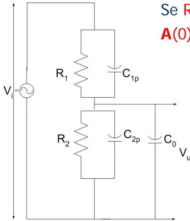
Se  $R_2 C_2 = R_1 C_{1p} \Rightarrow C_2/C_{1p} = R_1/R_2 \Rightarrow$
